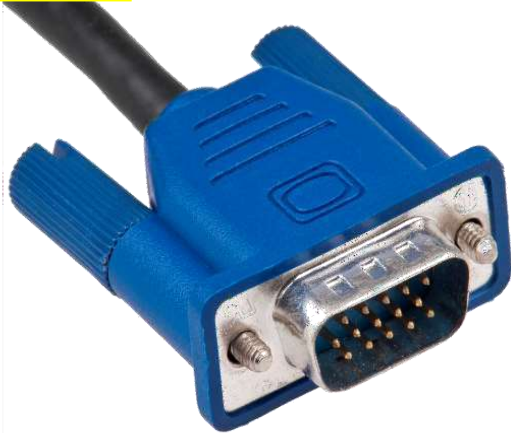
VGA cable with DE-15 male connector VGA = Video Graphic Array
