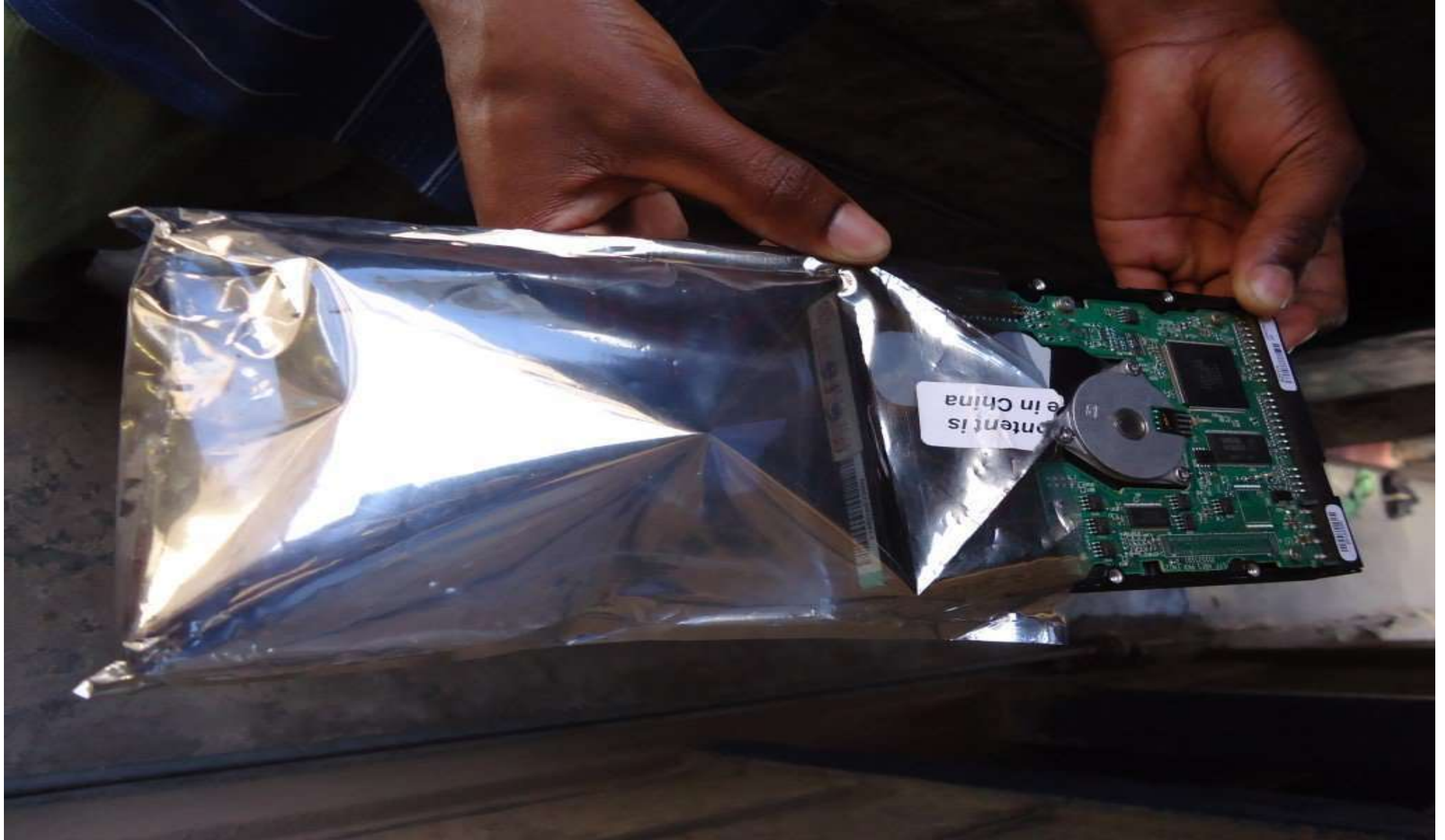
A hard disk drive (PATA type)
