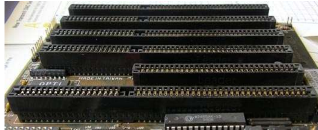
One 8-bit and five 16-bit ISA slots on a motherboard
